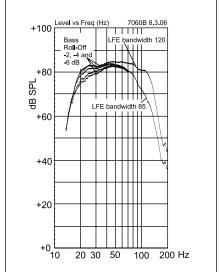
Figure 9. The free field frequency response of the 7060B subwoofer at different Bass Roll-Off settings
